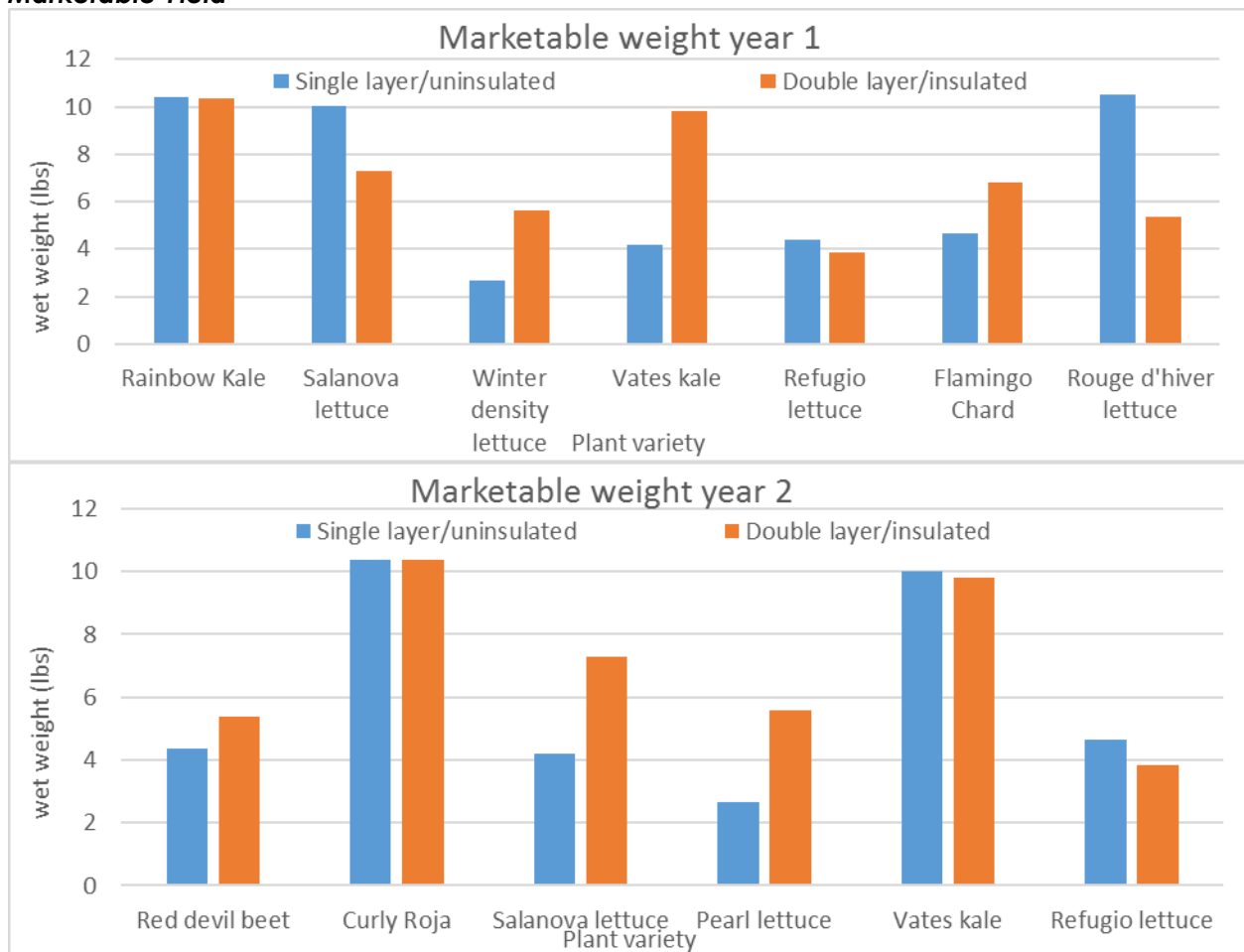
Figure 8: Comparison of plant marketable weights from year one and two of this study in single layered un-insulated greenhouse (GH1) and double layered insulated greenhouse (GH2).
