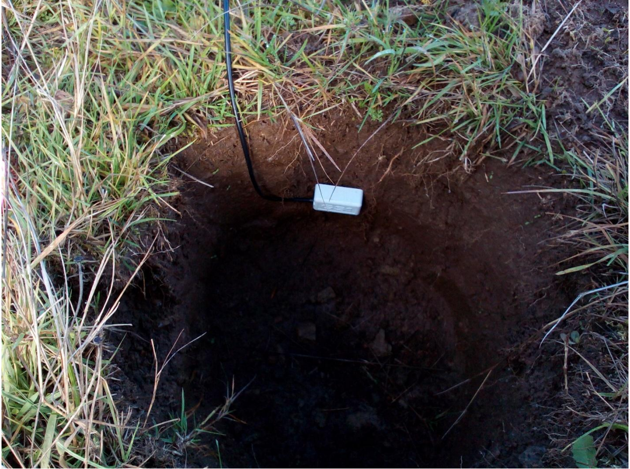
Photo 7 Installed Soil Moisture Probe at 10-cm Depth at Bullock Lake Farm
