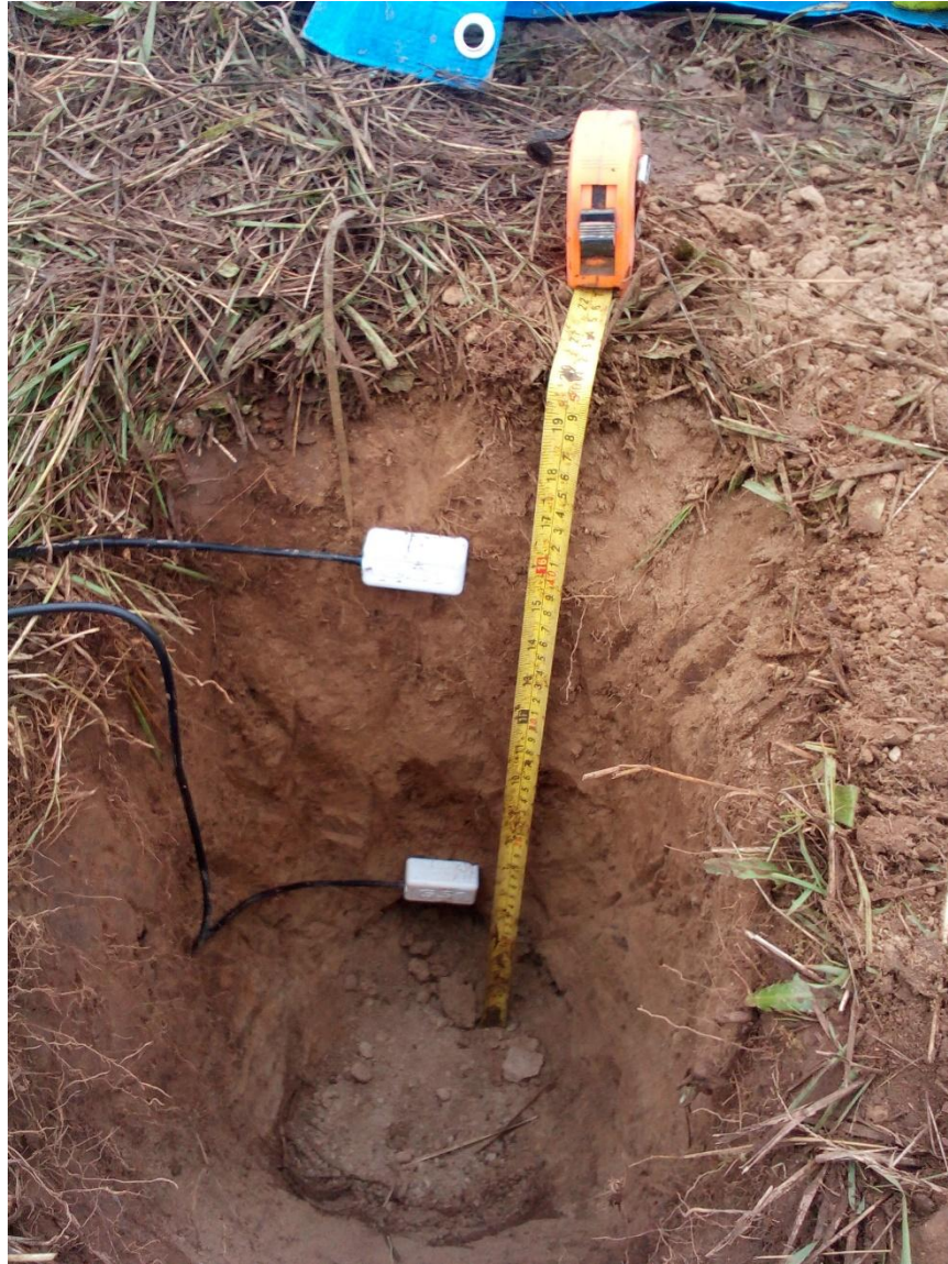
Photo 10 Installed Soil Moisture Probes at 10-cm and 40-cm Depths at Ravenhill Farm
